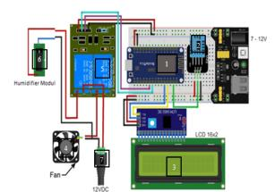
Figure 2. Initial Design of the Air Monitoring Device in the BSF Breeding Space
